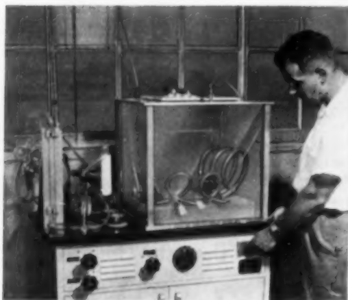
SAMPLES of Type AB insulated cable bent in small circles are placed in ozone chamber for ozone-resistance test.
